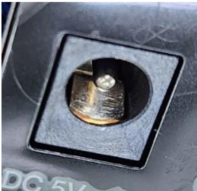
After cleaning DC connector GND
